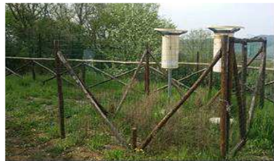
Figure 2 Example of installation Depobulk in the field
