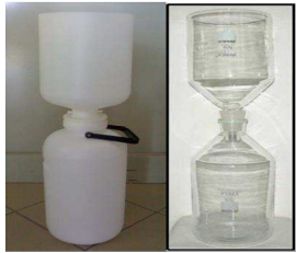
Figure 1 Material of depobulks, to the left in PHDE and to the right in Pyrex
