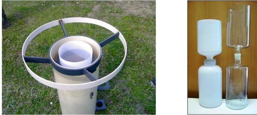
**Figura 6.2 - Deposimetri in vetro e in HDPE.**
